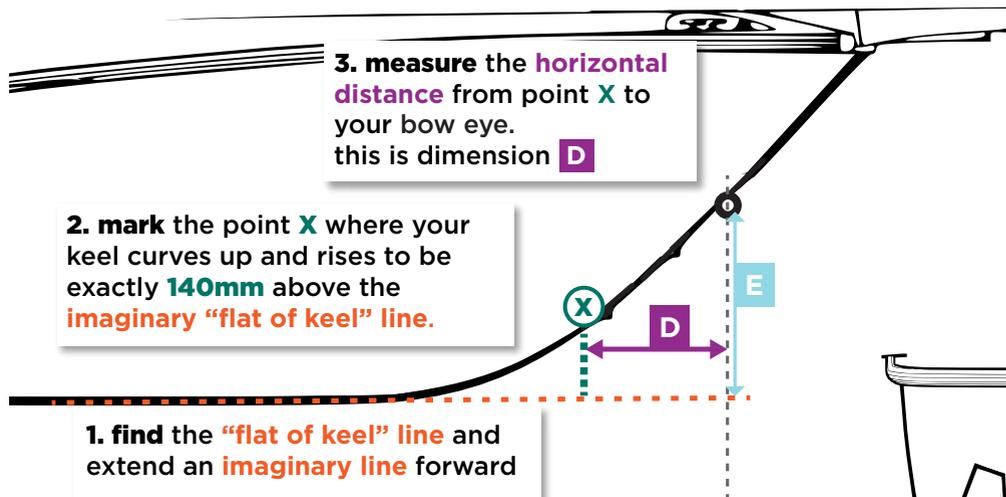
The top of the C-channel at the front of our trailer is 140mm higher than our keel slides, so we are finding the lowest point on your bow where your boat will still clear the C-channel. This determines how far forward we can bring your boat, and is required to calculate whether or not a trailer will fit.
